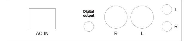
AC Power connection 240V / 230V / 220V / 115V / 100V AC dependent on country. Digital output Phono/RCA
